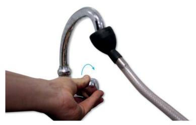
**10. Fill the kettle with cooling/heating water** Open the water valve that much that water connection stays on the valve.
