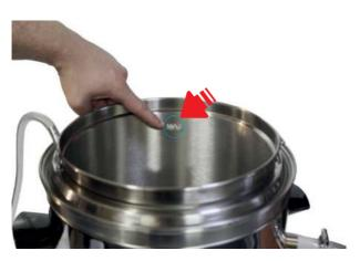
**5. Filling the milk container** Fill the milk container till mark "MAX".
