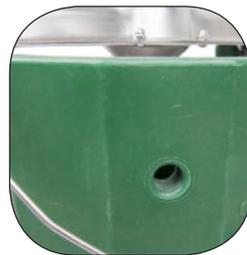
Keep the drain hole clear of ice to ensure the salty water does not get into the ice cream.
