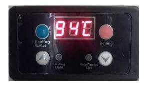
Temperature parameter represents the temperature of secondary water (heating water). <u>Temperature of milk is lower and must be measured separately!</u>
