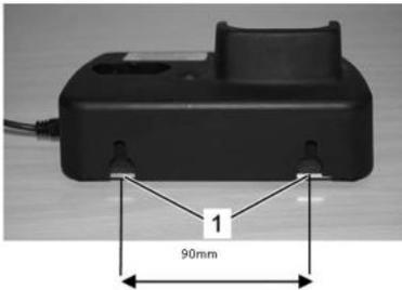
1. Place the charging station on a firm, even, dry, clean and free underground.
